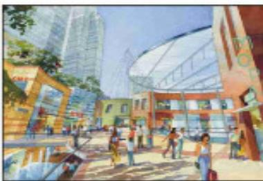
KLC provided schematic design of a three-dimensional roof system on top of one of the retail building. The span of the roof is approximately 40 meters and supported by twelve columns.
